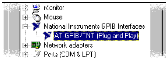
Figure 2-5. GPIB Interface That Is Working Properly
